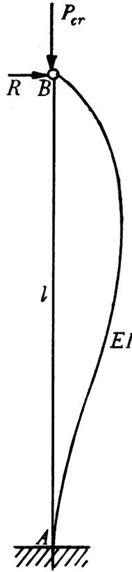
Fig. 1: Geometry of a bar with one end fixed and the other pinned under buckling conditions
